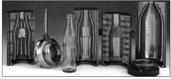
The temperature of the mold or plunger used to make glass containers is very critical to the quality of the glass container. If the mold is not cooling properly the container may exit the mold and not retain its shape or if too cool it will not be molded properly. The operators need to measure the molds to be sure the cooling is proceeding at the proper temperature.
