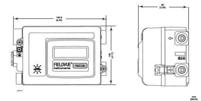
Figure 4. Dimensions for Type DVC2000 Digital Valve Controller
