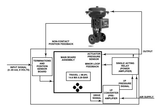
Figure 3. DVC2000 Series Digital Valve Controller Block Diagram
