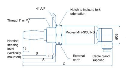
It's simple to order. Just choose from the 6 process connections with either direct load switching or PNP/PLC switching output. For example, a 3/4" BSPT threaded version to be used for switching a load: order the VT00.
