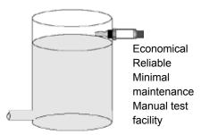
Many processes are controlled by plant computers, and tank levels are often measured by transmitters. It is common practice to fit an independent high level alarm switch to provide extra back up to the transmitter in case of failure.
