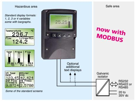
The BA484D is an intrinsically safe instrument that can display text and simple graphics in a hazardous area. Incorporating six push-buttons and two solid state outputs, the BA484D is a low cost operator interface ideal for simple machine and process control applications. Incorporating Modbus, BEKA and Legacy protocol the instrument may be used for new installations or to upgrade existing intrinsically safe systems.
