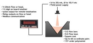
DM3600 can be used with almost any level sensor to measure "head" upstream of a flume or weir. Standard software allows power 3/2 and 5/2 flow linearisation, giving a (4 to 20) mA output proportional to flow, as well as pulsing a relay in multiples of flow rate to an external totaliser.
