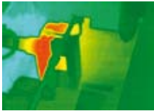
Motor: Bearing Problem
